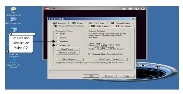
ETR recommends DVD Quality for encoding, especially where the video contains a lot of motion, but remember good quality digital video uses up more hard drive space. Use Good Quality where the video has less motion to preserve VOD Server storage space.
